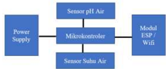
Gambar 2. Diagram blok node sensor
